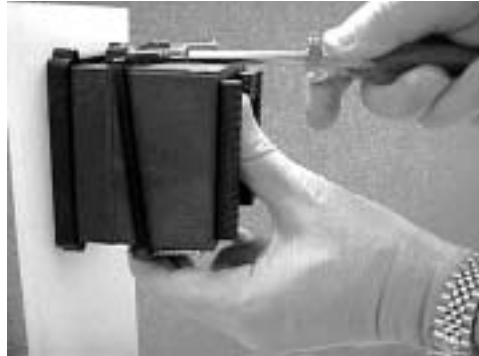
Figure 8.4 — Disengaging the Mounting Bracket.
