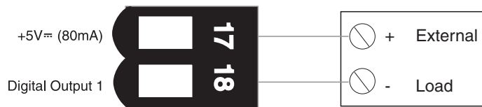
Figure 12.9c — Switched DC Example
