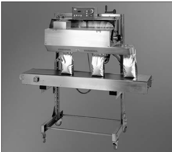
Audion Model 555 Adjustable Head Band Sealer shown with optional conveyor.
