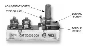
heated surface, a temperature change is sensed almost instantaneously. With an incrase in temperature, the case expands. This results in a linear change of the internal bridge assembly causing the electrical contacts to open. A decrease in temperature closes the contacts.
