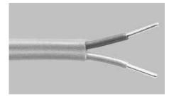
A relatively new fluoroplastic, PFA, is the insulation on SERIES 516. PFA's temperature rating is only slightly less than TFE. However, PFA can be applied using conventional extrusion techniques. This produces a smooth finish, as opposed to the spiral usually associated with TFE tape constructions. This is important in the food industry where taped constructions present cleaning problems. The smooth surface also allows this construction to be pulled through conduits and cut-outs more easily.
