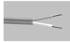
The SERIES 507 is the most economical fluoroplastic insulated wire. SERIES 507 is also available as UL® listed PLTC. Individual conductors are coated with a layer of color coded FEP. The insulated conductors are then parallel duplexed with an additional layer of color coded FEP. The finished construction has a temperature rating of 260°C (500°F). Abrasion, moisture and chemical resistance are far in excess of most other insulations.
