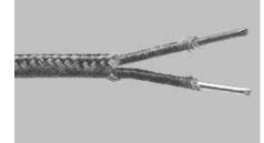
SERIES 305 is specifically constructed for light duty applications where size is a critical factor. The single conductors are insulated using a specialized yarn wrapped on the conductors in layers. This yarn is then impregnated to add abrasion resistance and enhance electrical properties. The insulated single conductors are then laid parallel and covered with a layer of braided glass. A final impregnation is applied to the braid.
