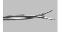
SERIES 511 is the most economical polyimide taped construction. The polyimide film applied to the conductors is considered to be the ultimate "soft" insulation. The tape maintains its strength at temperatures to 315°C (600°F). The FEP laminate serves as a moisture barrier and allows the tape to fused with itself. The finished construction will not unravel when cut.
