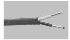
The primary and duplex insulation of SERIES 508 is fused TFE tape. The tape is spirally applied to the conductor and heated. This process, called sintering, forms the tape into a homogeneous layer. When sintered, the tape exhibits all of the advantages of extruded TFE insulation, while eliminating the concentricity problems associated with TFE extrusions.
