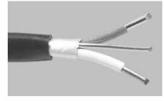
The SERIES 510 UL® is UL® listed for Power Limited Tray Cable (PLTC) applications. It's an economical PVC insulated, twisted and shielded construction for microprocessor based systems and others that are sensitive to induced voltages and "noise."
