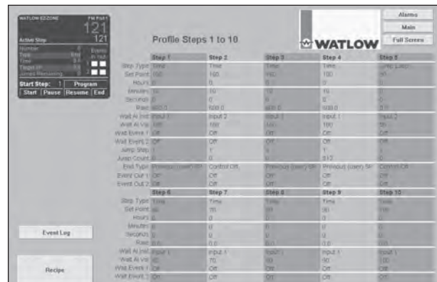
Make screens with most often used parameters. Enable recipe management to reduce operator errors when setting values.
