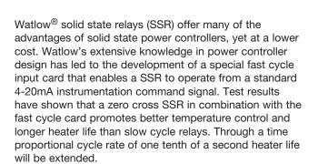
Both low and high voltage models are available from 24 up to 530VAC. All ac output models include back to back Silicon Controlled Rectifiers (SCRs) for a more rugged design than the traditional triac based SSR. The internal design allows it to handle high currents and the harsh electrical environments of heavy industry. Watlow also offers a switched VDC model for dc heating applications.
