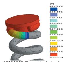
MICROCOIL Thermal Analysis using ANSYS® DesignSpace®
