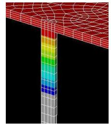
**Straight Thermocouple Thermal Analysis**
